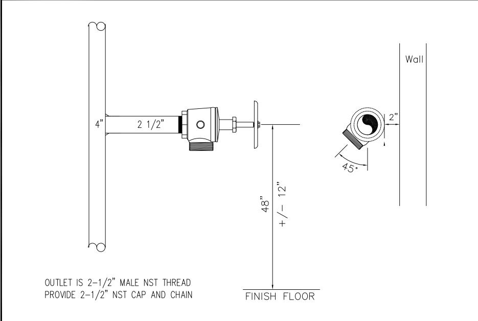
HOSE STATION SHALL BE MARKED TO INDICATE THE USE. LETTERS SHALL BE RED WITH A WHITE BACKGROUND AND BE 2-1/2" IN HEIGHT.
